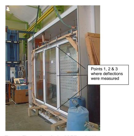
Figure 1. The specimen in the BRE Test rig 'G'
